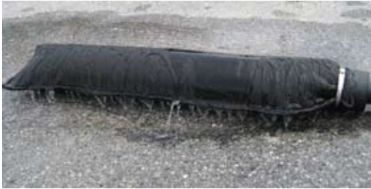
EVAC Filtration System filtering water.
