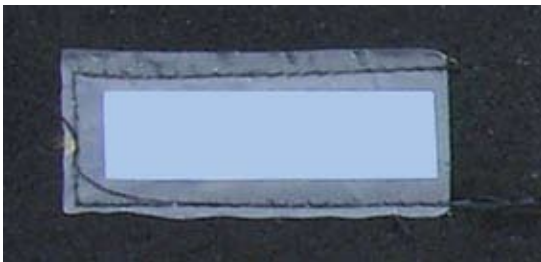
Oil Test Paper placed against outer layer.
